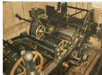
The clock mechanism is in three parts. On the left is the chiming mechanism; on the right is the hourly striking mechanism and in the middle is the clock mechanism.
